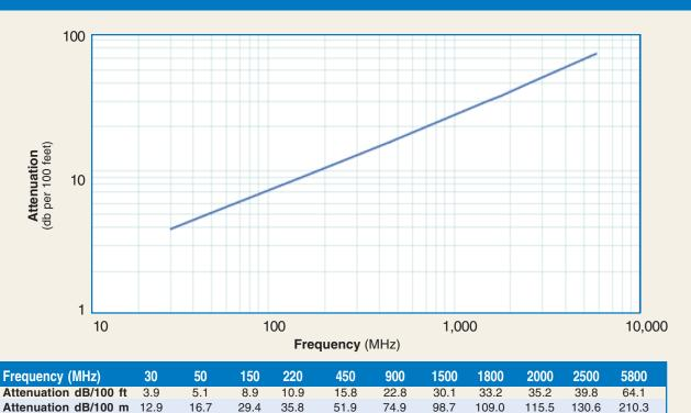
Calculate Attenuation = (0.709140) • √FMHz + (0.001740) • FMHz (interactive calculator available at http://www.timesmicrowave/telecom)
